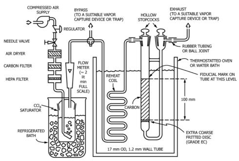
Note 1—These items for the apparatus are critical: the dimensions of the sample tube; the location of the flowmeter downstream of the  $CCl_4$  saturator; and the location of the stopcocks. Reheat coil must be adequate to bring the gas temperature to within 1 °C of the water bath temperature (that is, bed temperature).
